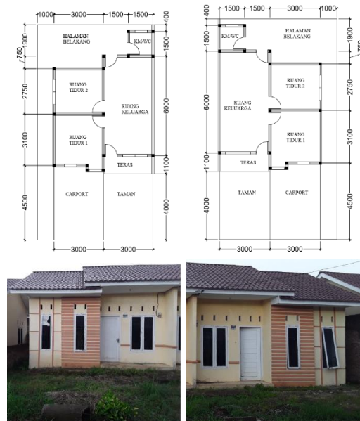
Figure 2. Initial plan and front view of the subsidized house for Grand Permata Residence II Housing, Deli Serdang Regency
