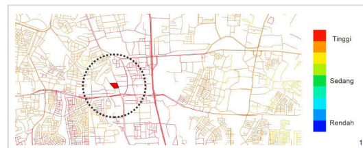
Figure 1. Axial map of the integration value of the area surrounding the Jatinegara Barat flats
