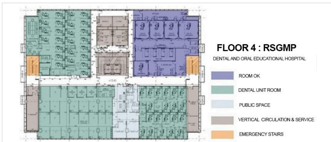
Figure 19. On the 4th floor, space zoning is in accordance with its functional designation, namely RSGMP based on temperature and relative humidity
