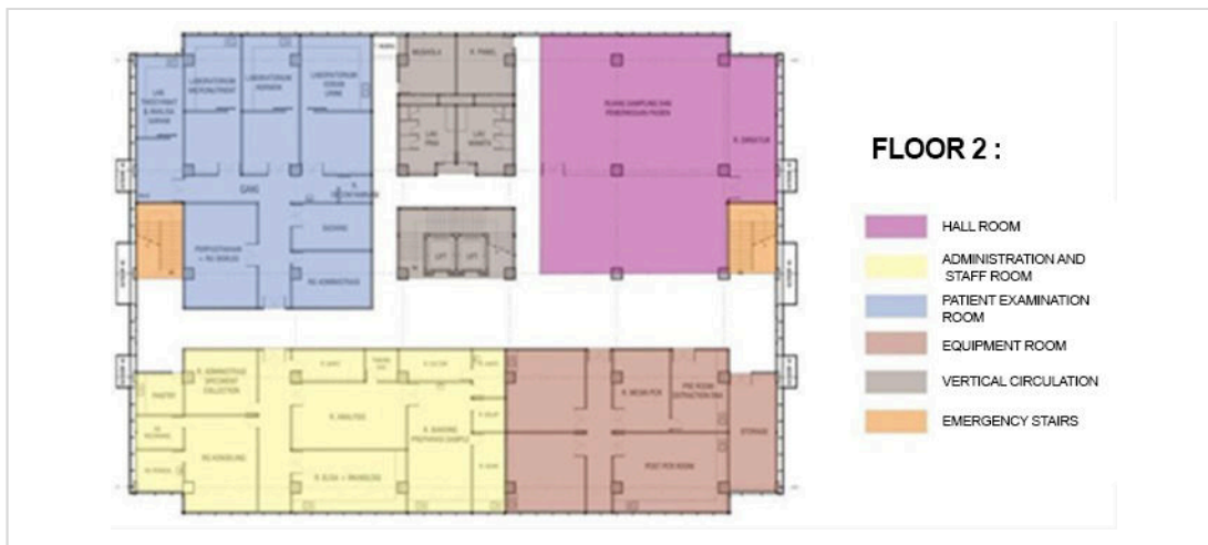
Figure 17. On the 2nd floor, public spaces such as halls, administration and patient examinations are recommended which can make things easier for users
