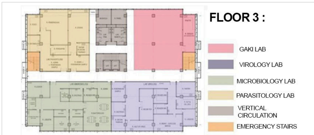
Figure 18. On the 3rd floor, all laboratories are focused on one floor to suit the temperature and relative humidity where the area allows for this function
