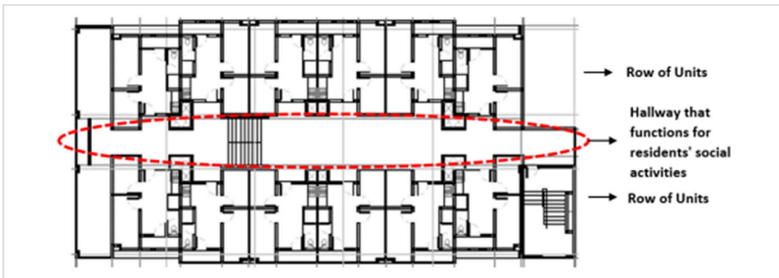
Figure 7. Typical floor plan of one building block in Akuarium Vertical Kampong Source: Ashadi et al. 2021
