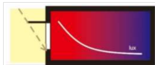
Figure 2. Unilateral side opening position using horizontal shading device Source: (Lechner 2015)
