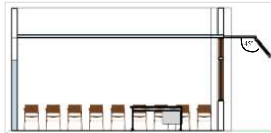
Figure 10. Section of classroom with 45^\circ shading device
