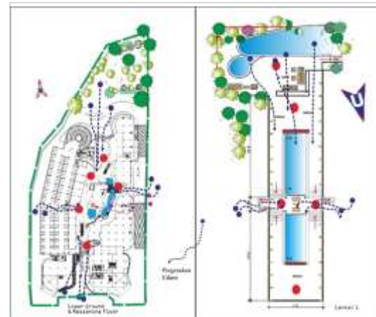
Figure 13. Air movement and wind speed measurement points at Nipah mall and Maxone hotels
