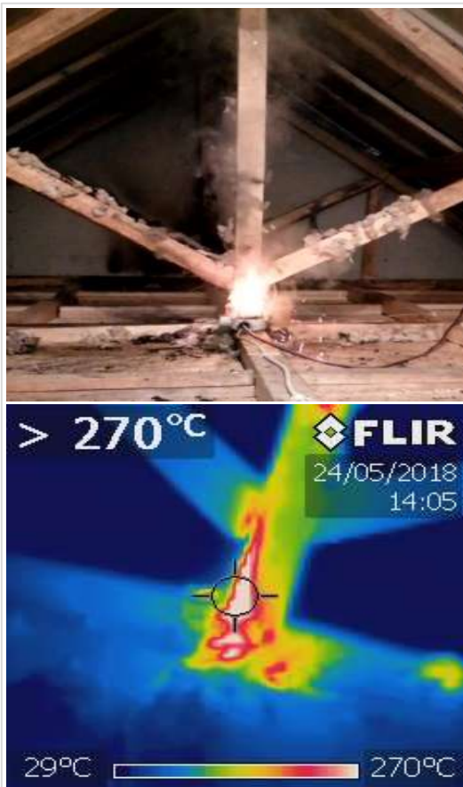
Figure 10. Analysis result of the gable roof model, with the fire source located at the centre of the room. The ignition stage began at 02.05 p.m. with a temperature of 270 °C. Ignition occurs in the 4th minute
