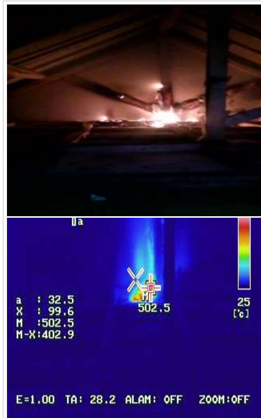
Figure 13. Analysis results of the gable roof model, with the fire source located at the edge. The flashover stage started at 09:26 a.m. with a temperature of >500 °C. Flashover occurred in the 9th minute
