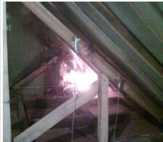
Figure 16. Analysis results of the shed roof model, with the fire source located in the corner of the room. Ignition stage began at 09:56 a.m. with a temperature of 430 °C. Ignition occurred in the 4th minute
