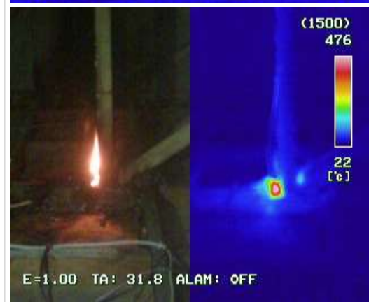
Figure 18. Analysis result of the shed roof model, with the fire source located in the centre of the room. The ignition stage began at 01:02 p.m. with a temperature of 442 °C. Ignition occurred around the 3rd minute
