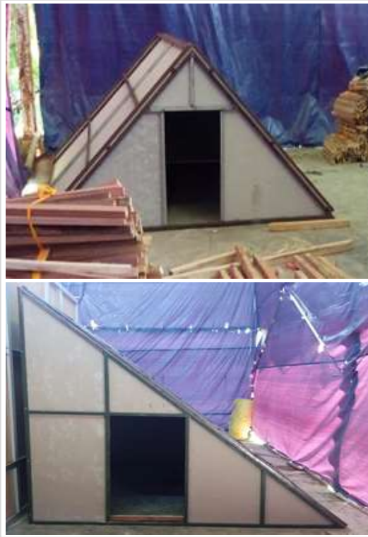
Figure 5. Scaled models of a gable roof (above) and shed roof (below)
