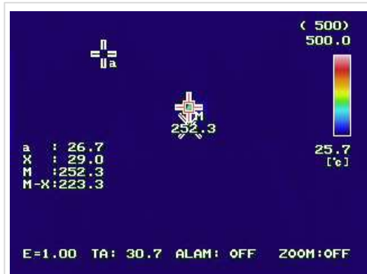
Figure 12. Analysis result of the gable roof model, with the fire source located at the edge. The ignition stage began at 09:23 a.m. with a temperature of 252 °C. Ignition occurred in the 6th minute
