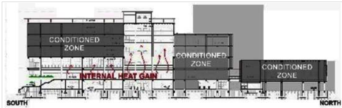
Figure 10. Lobby and atrium using natural ventilation
