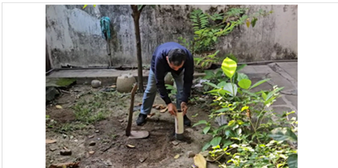
Figure 1. Samples of soil for the permeability test procedure
